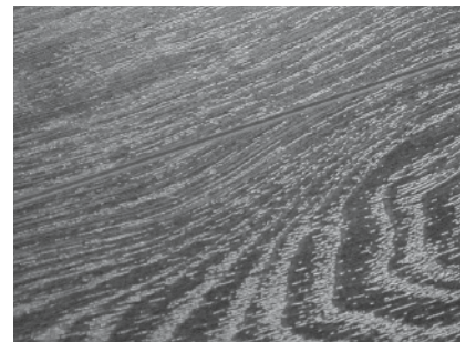
ER (registered emboss): genuine wood appearance due to consistence between pattern and embossing
